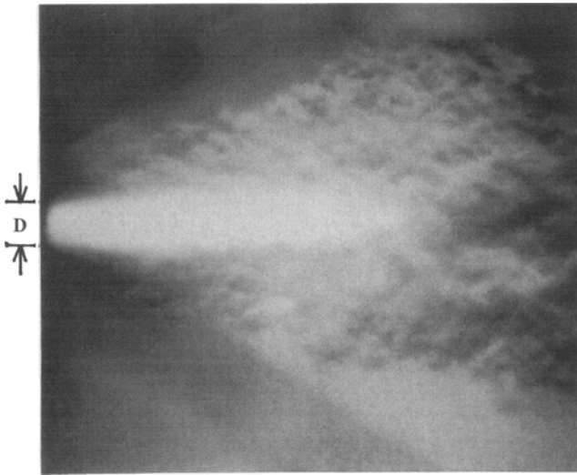
Fig. 2(b) Near-field of the GSP jet showing the large region of ambient fluid affected by the plasma jet. Same operating conditions as in Fig. 2(a).
