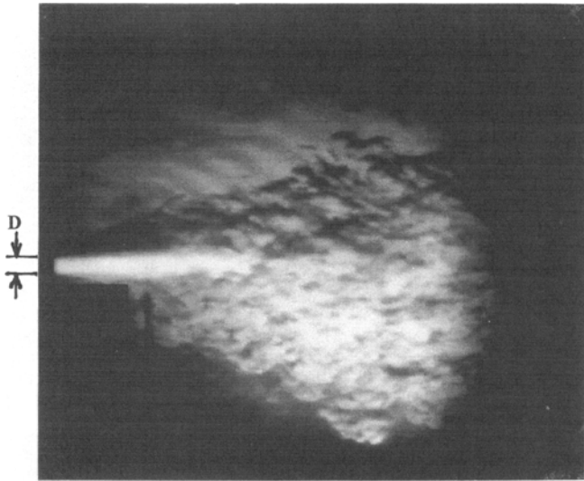
Fig. 3(a) Schlieren image of the WSP jet with an arc power of 160 kW
